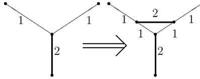
Fig. 6.  $(Y \rightarrow \Delta)$  operation.
